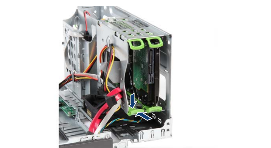
Figure 30: Inserting the Easy rails
